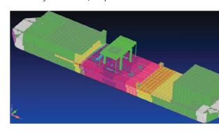
"VeriSTAR Hull is an extensive customization of Femap, designed to reduce the time required to generate finite element models as well as postprocessing."
