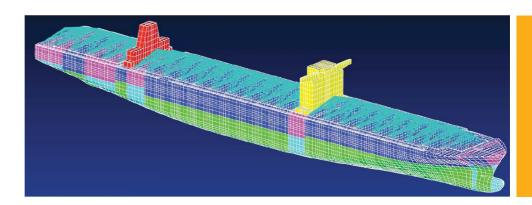
The ease of customizing Femap enables Bureau Veritas to keep its ship hull verification tool up-to-date with the latest versions of international rules
